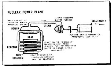
The main difference between a conventional steam power plant (top) and a nuclear plant lies in the source of heat used to make the steam that drives the turbines. In the reactor (bottom), heavy water flows over hot uranium rods and becomes hot itself. It is then pumped through a boiler (heat exchanger) where it gives up its heat to ordinary water that is converted into steam.
